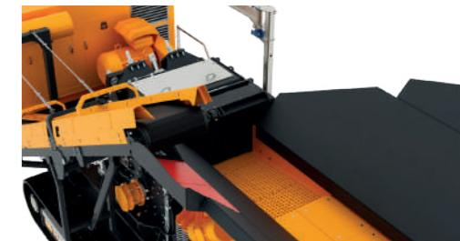
Wear-resistant plate feeder + intermediate screen
