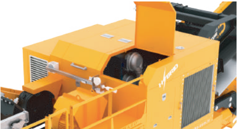
Easy Access to Engine Compartment
