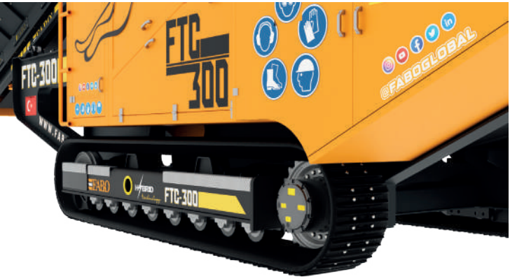
Track System: Provides superior mobility and stability on rough terrain.
